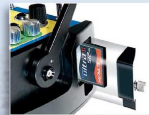
Measurement report, reloading of additional rail references and software updates via removable media (CF-Card)
